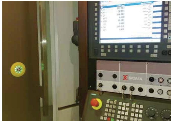
EAO's Series 56 (yellow, left side) is used in the redesigned control panels.
