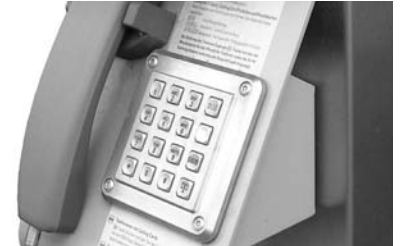
Where switch controls are used determines the degree of environmental protection necessary.
