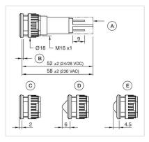
A = Protection tube (only 230 VAC) B = 1 gasket C = flat conical D = round
