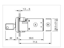
$\label{eq:approx} A = Screw terminal \\ B = Plug-in terminal 6.3 mm x 0.8 mm$
