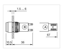
A = Solder terminal B = Plug-in terminal 2.8 mm x 0.5 mm
