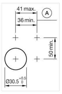
A = Action range of aligning pins
