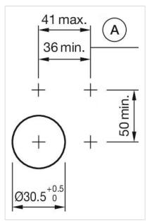
A = Action range of aligning pins
