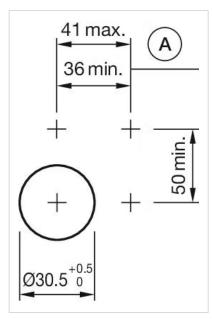
A = Action range of aligning pins
