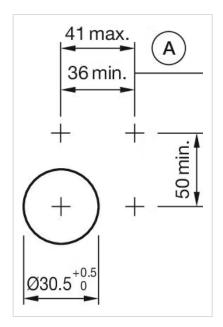
A = Action range of aligning pins
