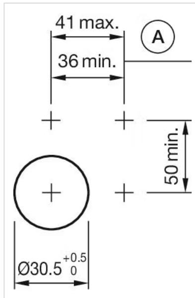
A = Action range of aligning pins
