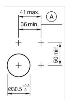
A = Action range of aligning pins
