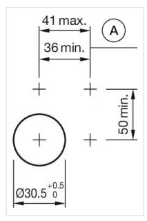
A = Action range of aligning pins
