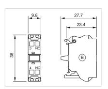
B = Spring-type terminal for Part No. 45-311.1Z40, 45-311.1X40
