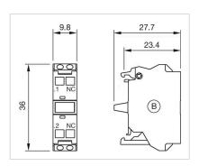
B = Spring-type terminal for Part No. 45-312.1X40
