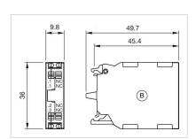
B = Spring-type terminal for Part No. 45-314.1X40
