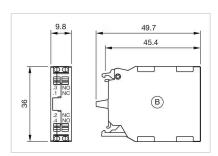
B = Spring-type terminal for Part No. 45-315.1Z40, 45-315.1X40
