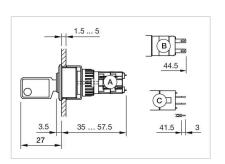
A = Solder terminal B = Solder terminal 2.8 mm x 0.5 mm C = Universal terminal 2.0 mm x 0.5 mm
