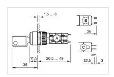
A = Solder terminal B = Plug-in terminal 2.8 mm x 0.5 mm C = Universal terminal 2.0 mm x 0.5 mm
