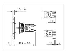
A = Solder terminal B = Plug-in terminal 2.8 mm x 0.5 mm C = Universal terminal 2.0 mm x 0.5 mm
