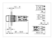
A = Solder terminal B = Plug-in terminal 2.8 mm x 0.5 mm
