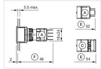
$\label{eq:Absolute} A = \mbox{Plug-in terminal } 2.8 \mbox{ mm x } 0.5 \mbox{ mm} \\ C = \mbox{Screw terminal}$
