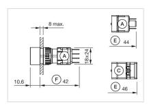
A = Plug-in terminal 2.8 mm x 0.5 mm C = Screw terminal
