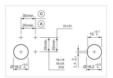
A = Solder/Plug-in terminal 2.8 mm x 0.5
