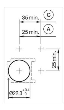
A = Solder/Plug-in terminal 2.8 mm x 0.5
