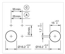
A = Solder/Plug-in terminal 2.8 mm x 0.5
