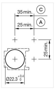
A = Solder/Plug-in terminal 2.8 mm x 0.5 mm
