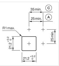
A = Solder/Plug-in terminal 2.8 mm x 0.5 mm C = Screw terminal
