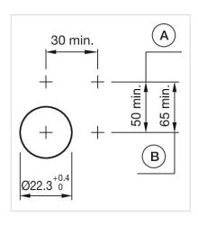
A = Screw terminal B = Push-in terminal (PIT)
