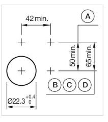
A = Screw terminal B = Push-in terminal (PIT) C = Plug-in terminal 6.3 mm x 0.8 mm D = Double plug-in terminal 6.3 mm x 0.8 mm
