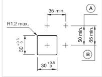
A = Screw terminal B = Push-in terminal (PIT)
