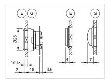
E = Lens raised above bezel G = Lens convexe raised above bezel
