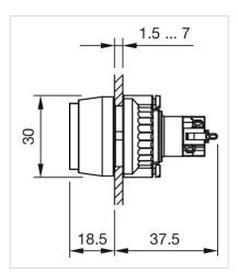
Illuminated pushbutton, Momentary, 250 V AC @ 3 A, 24 V AC/DC, 1 NC / 1 NO, Soldering terminal, Round, Green, Green
