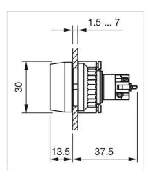
Illuminated pushbutton, Momentary, 250 V AC @ 3 A, 28 V AC/DC, 1 NC / 1 NO, Soldering terminal, Round, Blue, Blue
