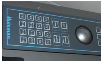
EAO's Series 70 switches are used behind the membrane for better levels of tactile feedback.
