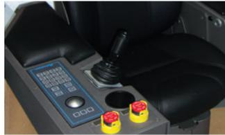
The panels include a trackball and membrane keypad for easy operation.
