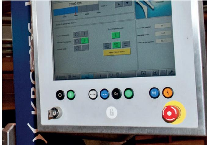
EAO also supplies KRONES AG with HMI Components, including pushbuttons and emergency stop switches.
